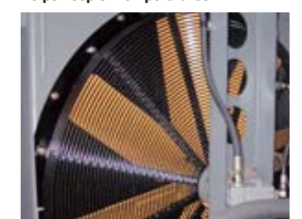
Strategically Positioned Oil Coolers— Helps keep oil temperatures
