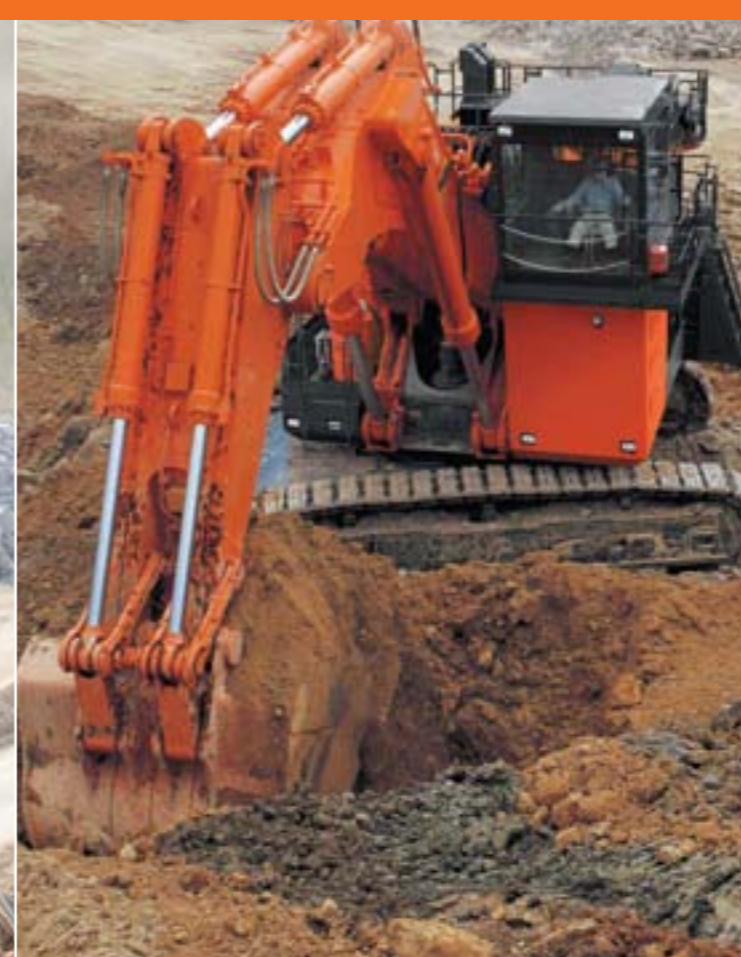
Rigid Box Design— Resists bending and twisting forces.
