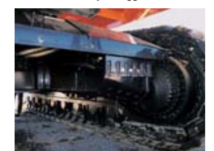
High-Mounted Compact Travel Motors and Optional Travel Motor Guard— Help to boost durability at rugged work sites.
